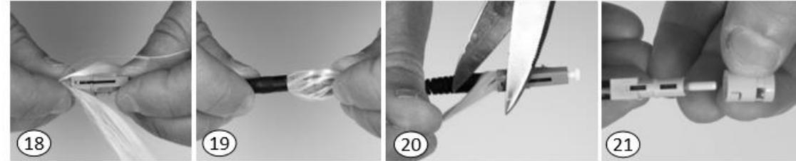
**5.9** Maintaining a slight force on the fiber (See **Figure 10**), release the wedge clip by squeezing both sides until the wedge clip dislocates itself from the connector body. Remove the wedge clip. (See **Figure 11**)
