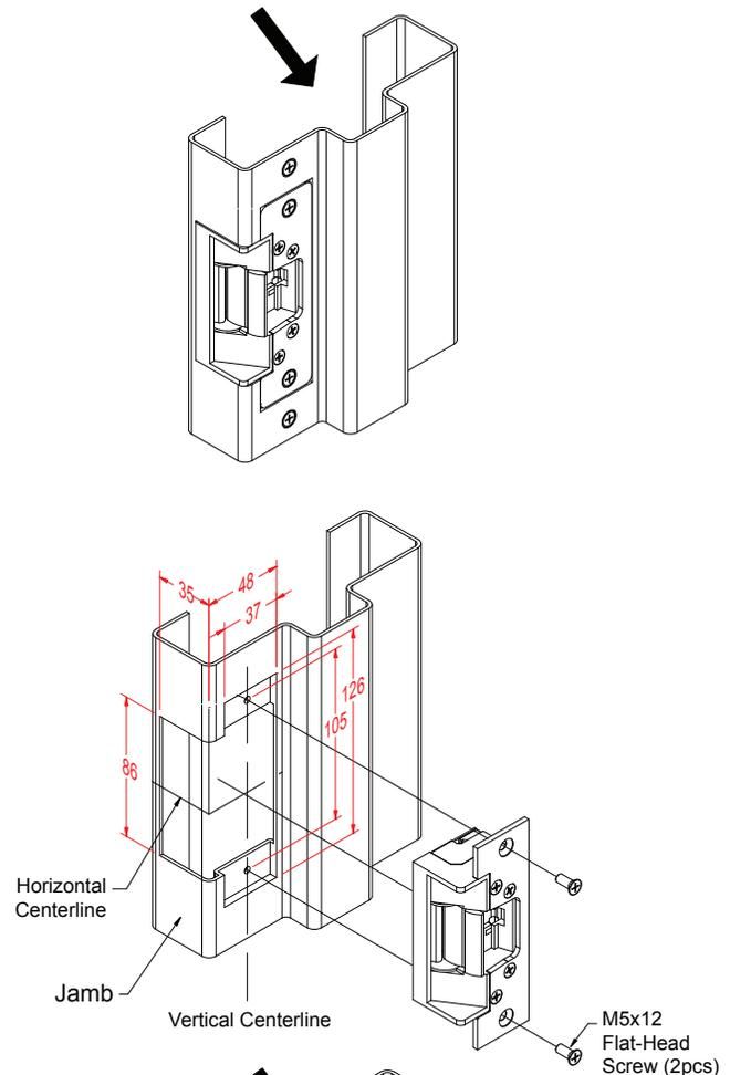
**Note:** The products are intended to be installed in accordance with the installation wiring diagram, mechanical assembly drawings provided with each product, the local authority having jurisdiction (AHJ) and the National Electric Code, NFPA 70. When installed in fail secure mode, the local authority shall be consulted with regard to the use of possible panic hardware to allow emergency exit from the secure area.
