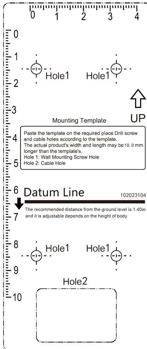
**Figure 3-5 Mounting Template**
