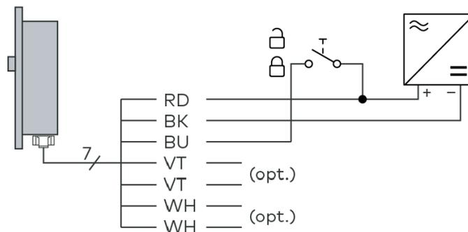
When in Fail Safe configuration, applying positive voltage to the control wire triggers the SL30SGL to lock (active-high locking signal). In the event of a power cut, the SL30SGL will unlock.
