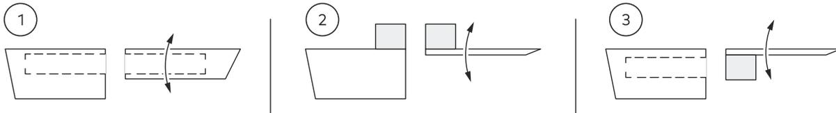
The lock and strike plate can be installed mortised (1), surface mounted (2), or a combination of the two (3). Regardless of the installation method it is vital that the lock face plate and strike plate are aligned vertically to each other and that the gap between them does not exceed 6mm (1/4 inch) when the door is closed.
